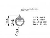
Hollow shaft with keyway. Use key 26062 or 26064. Material: Steel zinc plated. L=2750 mm. Material: Steel zinc plated. L=2750 mm.
